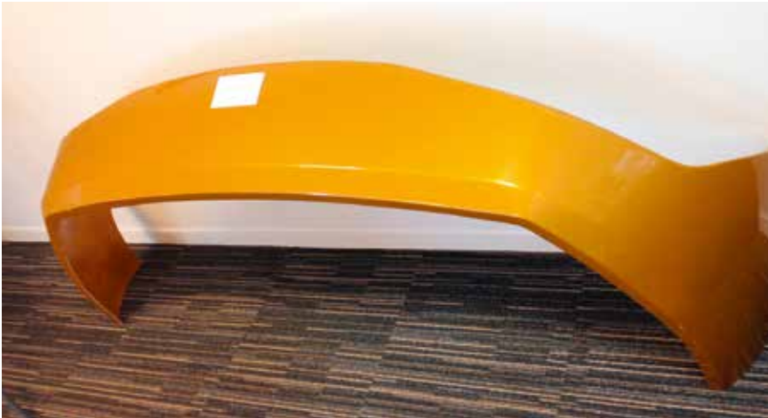
Fig. 2. Painted bus front end: The glass fiber composite was manufactured in cooperation with MVC Plasticos (© Arkema)
