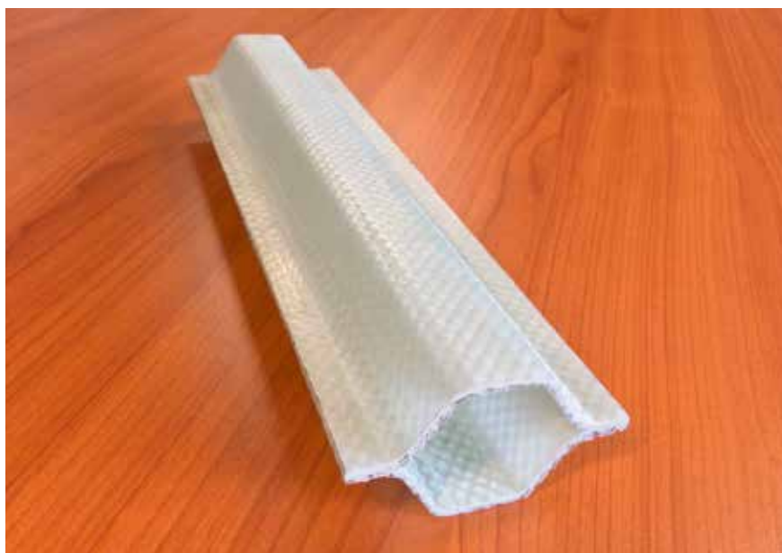
Fig. 1. Advantages of the thermoplastic acrylic resin: The composites can be thermoformed and welded (© Arkema)
